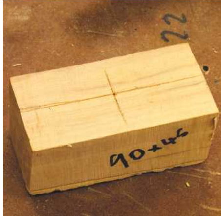
▲ Pic.20 The head of the hammer is the next thing to turn. Les has marked a line all the way round so he can drill the hole first and mark the centres accurately
